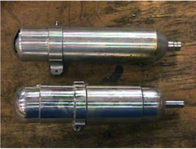
Pictured above is the prototype of the PDR0053 ProMuffler immediately below a Raptor 50 muffler.
