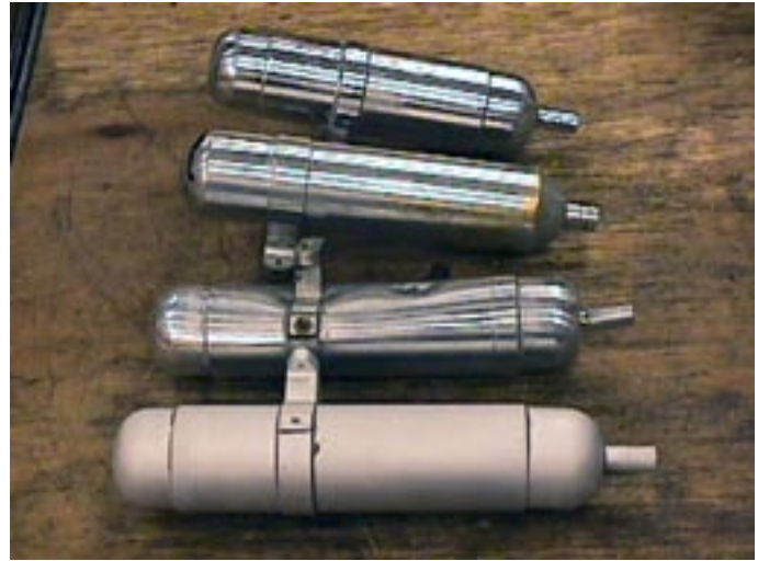
Variations on a theme . . . fater and longer! The V1 is at the top, then the Raptor 50 muffler, then other prototypes
