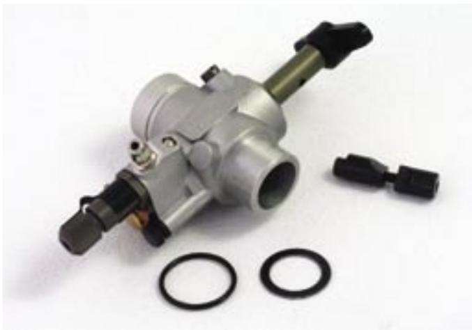
With the introduction of the superb 60L carburetor, the engineers at OS Engines gave modelers what may be the best all around 50-class carburetor on the planet! Superceding the 40E as used on the OS50SX-H, the 60L is used on the 50SX Hyper. Outwardly similar, the 10 mm the bore of the 60L carburetor is 1.5 mm larger in diameter than the 8.5 mm bore 40E carb.
