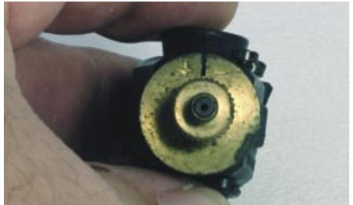
A disassembled Perry carburetor will lead you to understand why I compared it to the OS 60L carburetor. They share a similar design for achieving low-speed mixture. In the old days, though widely acknowledge for superb mixture control, some old timers didn't like how easily the tiny slot would get clogged by debris . . . I inturn became a master at the field stripping it!
