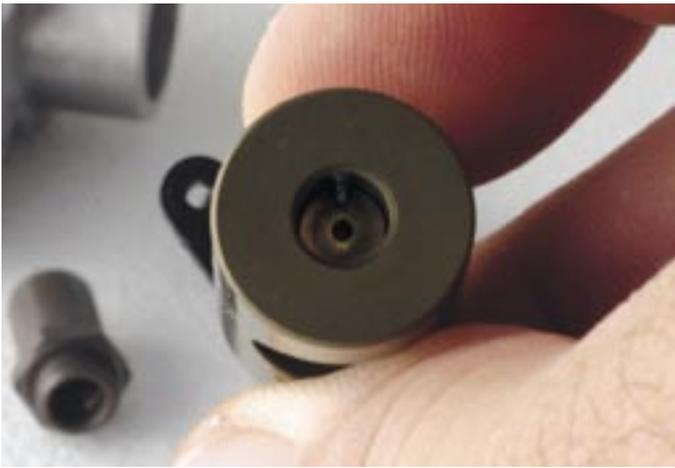
assembly so that you're looking at the end of the throttle barrel where you'll see the steel pin serves another function besides providing a stop for the spray assembly. This pin also serves to locate the little piece of the mixture assembly I call a cat's eye (for lack of a better word). I call it this because of the cat eye shaped slot machined at one end.
