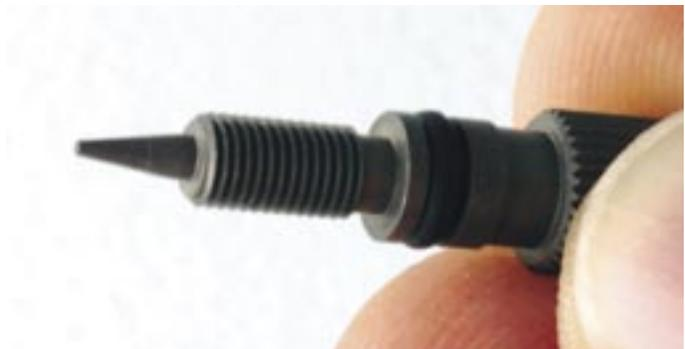
6. Using the 8 mm wrench to loosen it, remove the main needle assembly (where the main needle screws in). This is another prime candidate for trouble as it may hold trash which made it past the fuel filter.
