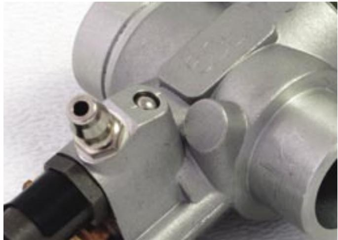
4. Note the steel ball pressed into the carb body. It's held in place when surrounding aluminum was deformed with a punch. Removal of this ball is beyond the scope of this white paper and regardless, isn't necessary since it's merely plugging a hole drilled for manufacturing purposes.
