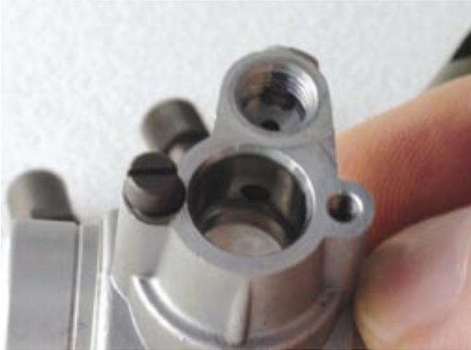
The above photo also illustrates the cam-action of the mixture control assembly perfectly. As you can see, it's machined in such a way that as you rotate it, the eccentric body of the screw serves to adjust the rotation of the brass mixture assembly.
